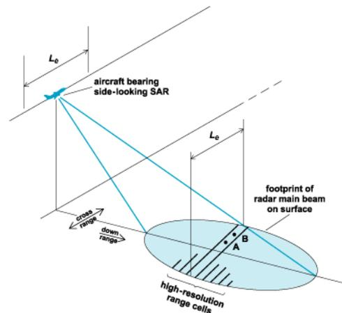
Figure 1 - Geometry of Example RADAR
