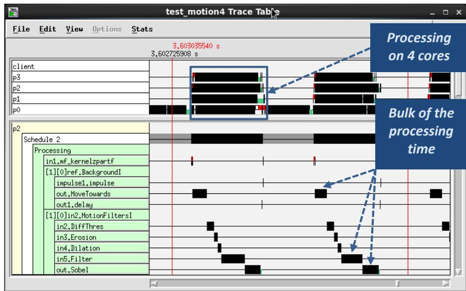
Figure 6 - Execution trace showing all events on all CPUs in the system
