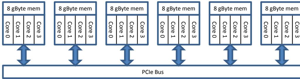
Figure 3 - Architecture of StarVX System
