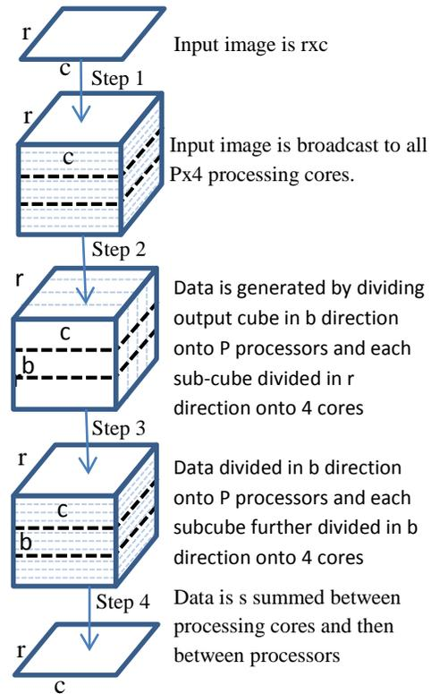
Figure 10 - Decomposition of data tokens for parallel processing
