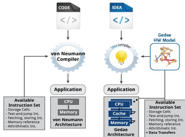
Figure 4 - The differences and similarities between the von Neumann and Gedae programming models
