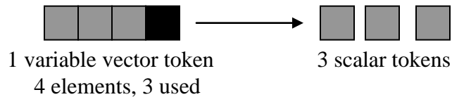
Figure 17 – Conversion from variable vector to scalar
